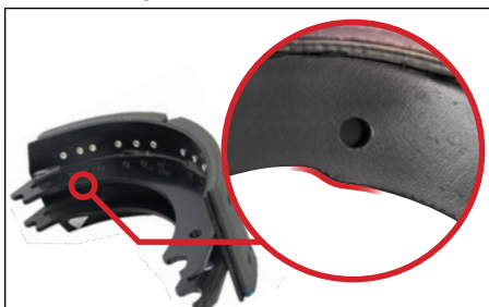
Q-style shoe with hump near pin hole.
