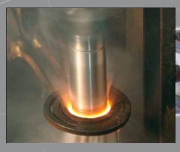
High carbon 45HRC toolgrade steel is used for all cam heads and journals Heat-treated cam heads run longer
