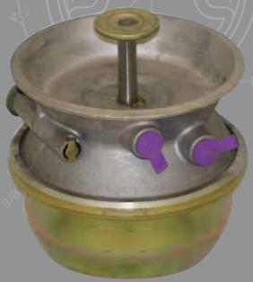
Non-reinforced chambers will disfigure under high pressure compounding and eventually compromise the pan integrity, causing "pull through" and ruining the unit.
