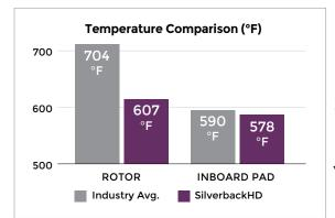
SilverbackHD pads keep the rotor temp. around 100 degrees cooler, resulting in longer service life.
