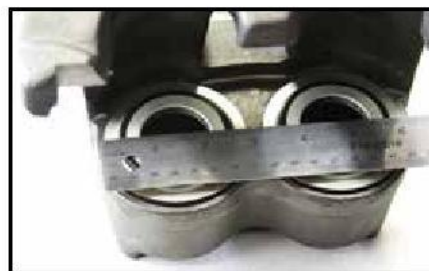
Piston Dia. Measurement
